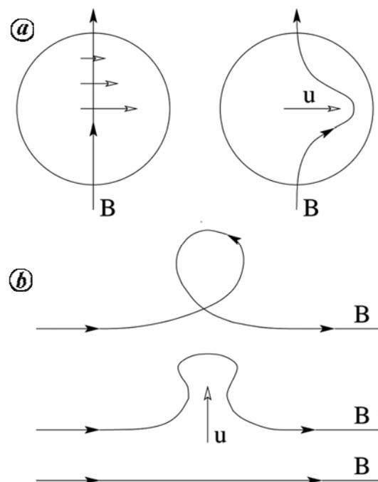
**Figure 1.** Schematic of the  $\alpha$ - $\omega$  dynamo cycle<sup>1,10,14</sup>. **a**, An initial poloidal field is swept by differential rotation to give a toroidal field; **b**, Fluid motion lifts and twists a toroidal field line to produce a poloidal field loop.
