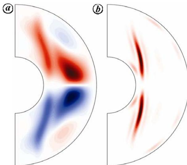
**Figure 6.** Azimuthally averaged meridional plots for a dynamo model at  $E = 5 \times 10^{-5}$ ,  $Ra/Ra_c \approx 6$ ,  $Pr = 1$  and  $q = Pm = 1$ . Positive values are shown in red and negative values in blue. **a**, Azimuthal magnetic field,  $B_\phi$ . **b**, Axial kinetic energy density,  $\frac{1}{2}u_z^2$ . No-slip, isothermal and electrically insulating boundary conditions are used. This model produces a stable, dipolar magnetic field.
